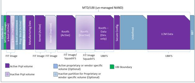
UBI is specifically designed for flash memory devices. Earlier bootloaders are not considered part of the UBI device because they are only responsible to interpret how U-Boot is formatted with UBI standard. Therefore, earlier bootloaders chain the bootloaders up until U-Boot from a raw flash device, bypassing the UBI layer entirely.
